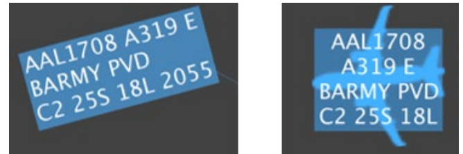
Fig. 2. Digital flight strips on the RTC display in the no metering condition: at the gate prior to pushback (left) and following pushback, while taxiing in the ramp area (right).
