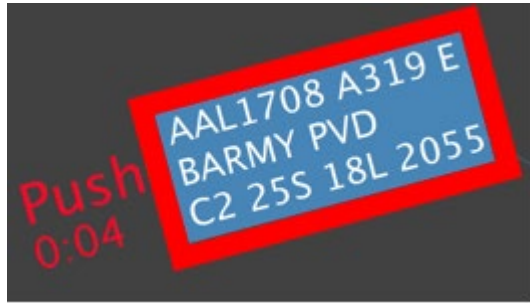
Fig. 4. The countdown timer begins to count up after the TOBT has been reached and the color of the time notification changes to red. Also, a red border appears around the flight strip to alert the Ramp Controller.
