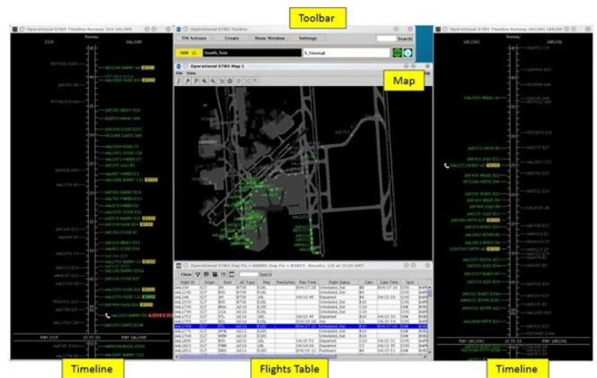
Fig. 6. The Surface Trajectory Based Operations (STBO) Client tool placed in the Tower, TRACON, and, in observer mode, in the Center.
